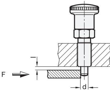
As soon as a gap *I* remains between the guide and the indexing bore hole opposite, the load can be reduced to a flexure rod clamped in at one side.
