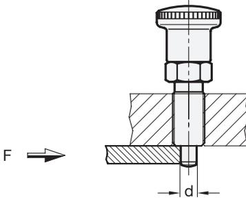
Provided that a miniscule gap remains between the guide of the indexing plunger and the indexing bore hole opposite, the load can be reduced to a clean shear action.
