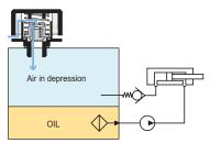
When in the reservoir a depression around 0.030 bar is produced, a flux of air entering the reservoir through the suction valve takes place.
