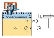
When in the reservoir an over pressure exceeding 0.350 (or 0.700) bar is produced, a flux of air is discharged through the safety valve.
